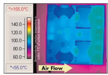
*Figure 6:* Thermal plot of converter at 60 amp load current with 55°C air flowing at the rate of 200 LFM. Air is flowing across the converter from input to output (nominal input voltage).
