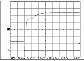
Figure 10: Turn-on transient at zero load (10 ms/div). Top Trace: Vout (0.5V/div) Bottom Trace: ON/OFF input (5V/div)
