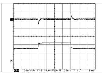
**Figure 12:** Output voltage response to step-change in load current (50%-75%-50% of Iout(max):  $dI/dt = 5A/\mu s$ ). Load cap:  $480\mu F$ , 15 m $\Omega$  ESR tantalum capacitor and  $1\mu F$  ceramic capacitor. Top trace: Vout (100mV/div), Bottom trace: Iout (20A/div).
