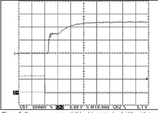
Figure 9: Turn-on transient at full load (resistive load) (10 ms/div). Top Trace: Vout (0.5V/div) Bottom Trace: ON/OFF input (5V/div)
