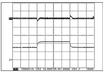
**Figure 11:** Output voltage response to step-change in load current (50%-75%-50% of lout(max);  $dI/dt = 0.1A/\mu$ s). Load cap:  $15\mu$ F, 450 m $\Omega$  ESR tantalum capacitor and  $1\mu$ F ceramic capacitor. Top trace: Vout (100mV/div), Bottom trace: lout (20A/div).
