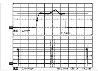
**Figure 18:** Load current (20A/div) as a function of time when the converter attempts to turn on into a 1 m $\Omega$  short circuit. Top trace (2.5ms/div) is an expansion of the on-time portion of the bottom trace.
