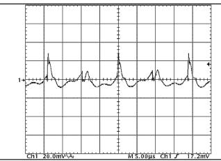
Figure 16: Output voltage ripple at nominal input voltage and rated load current (20 mV/div). Load capacitance:  $1\mu$ F ceramic capacitor and  $15\mu$ F tantalum capacitor. Bandwidth: 20 MHz. (See Figure 13)
