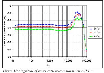
Figure 21: Magnitude of incremental reverse transmission (K1 –  $i_{in}/i_{out}$ ) for minimum, nominal, and maximum input voltage at full rated power.
