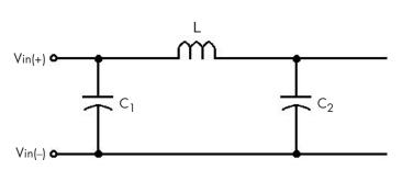
Figure E: Internal Input Filter Diagram (component values listed on page 3).
