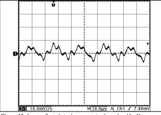
**Figure 15:** Input reflected ripple current,  $i_s$ , through a 10  $\mu$ H source inductor at nominal input voltage and rated load current (10 mA/div). (See Figure 13)
